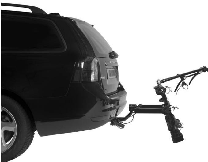
By pushing the entire carrier up, the tilting mechanism is locked again (you hear a click). Make sure to always secure the handle again by sliding this to the locking position.
